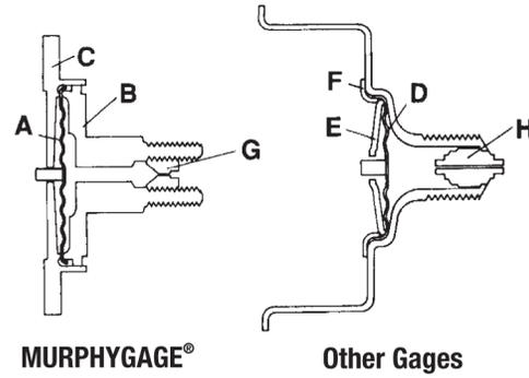
being used with liquids which might cause clogging. Other gages are usually equipped with a non-removable dampener (H).
