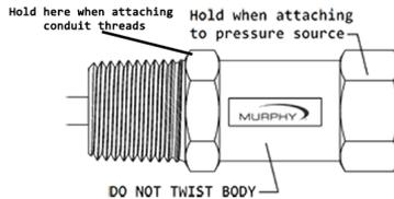
Transmitters require no special mounting hardware and can be mounted in any plane with negligible position error.
