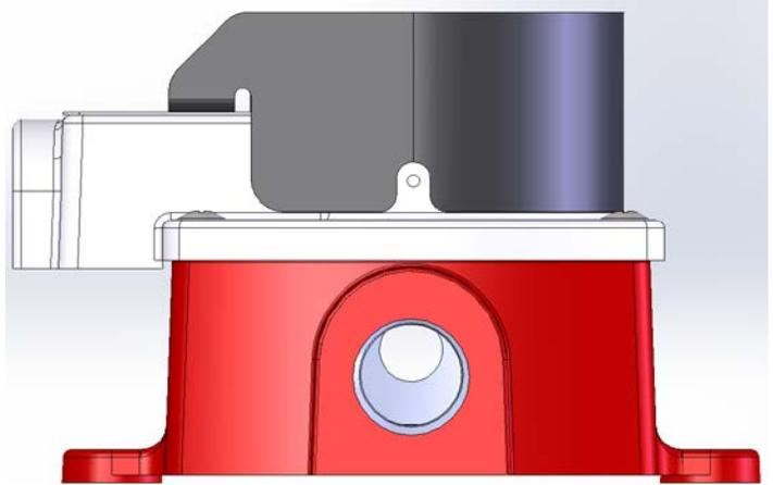
Align visor mounting holes with junction box cover mounting holes.
