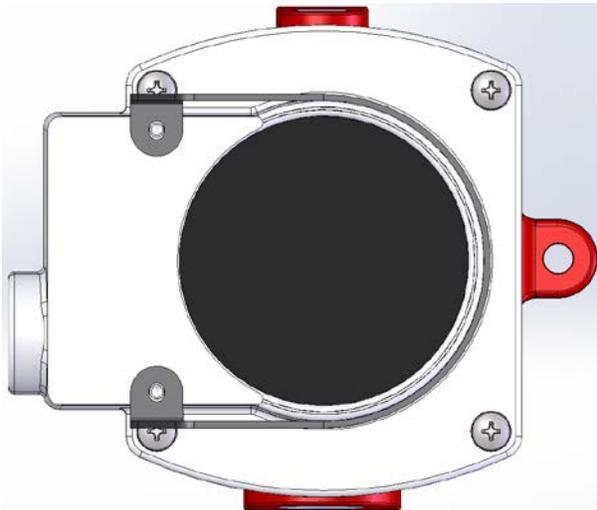
Install two screws supplied with visor, torque to 10 in. lbs.
